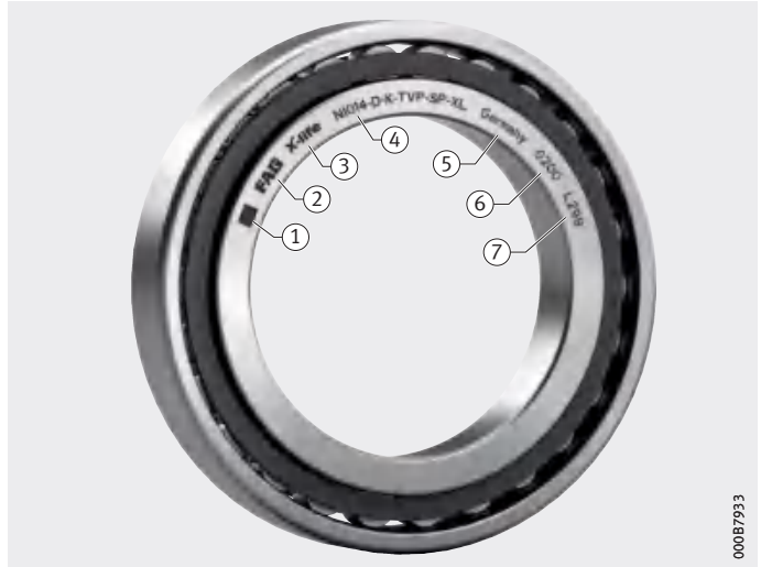
Figure 7 Example of marking for single row bearings with TVP cage
