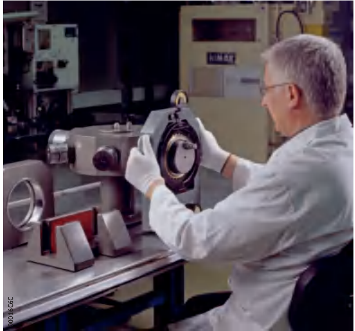
Figure 4 Positioning the enveloping circle gauge
