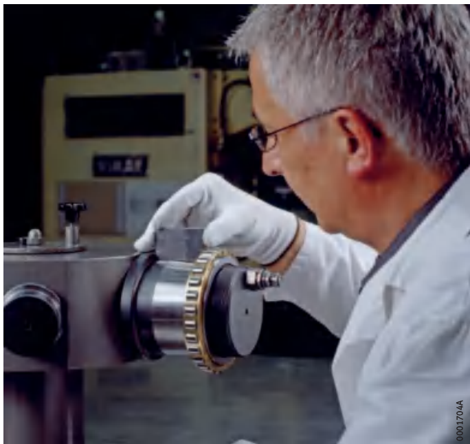
Figure 5 Measuring the spacing from the shaft shoulder
