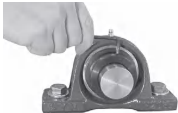
Fig. 14.10 Installing eccentric locking collar
