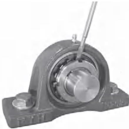
Fig. 14.8 Bending claw of washer (Locking locknut)
