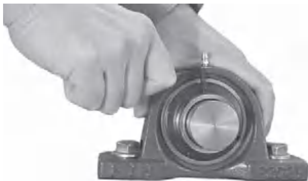
Fig. 14.5 Tightening of set screws
