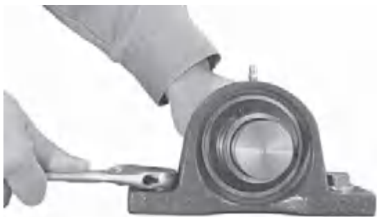
Fig. 14.4 Installation of setscrew units
