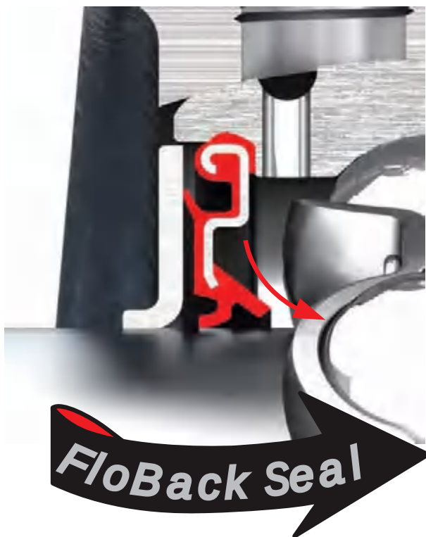
Fig. 1.3 Sealing mechanism of ball bearing units
