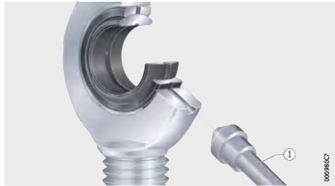
Figure 5 Relubrication via hole
