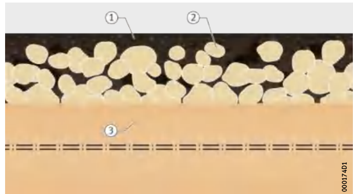
Figure 2 Maintenance-free plain bearing material E40-B
