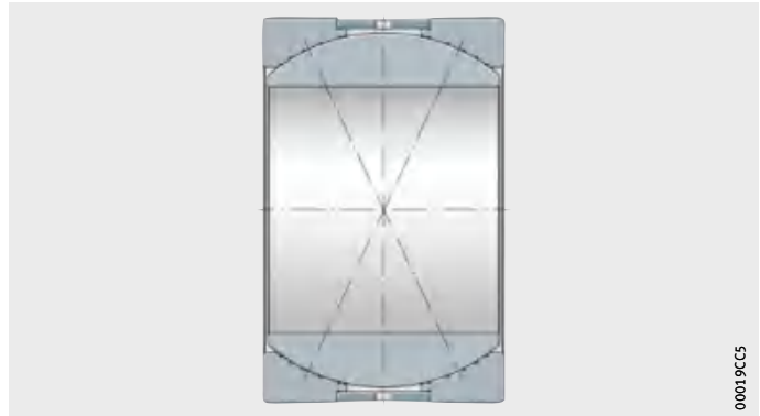
Figure 7 Locating bearing for articulated frame steering system
