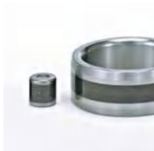
Fig. 17 Electric pitting generated on general purpose bearings (pits)
