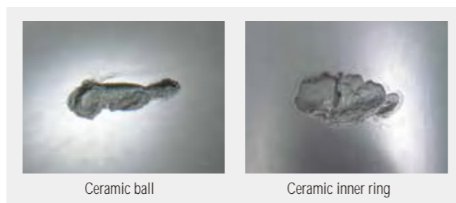
Fig. 6 Flaking on ceramic ball and inner ring
