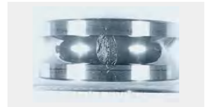
Fig. 13 Ceramic inner ring damaged by dynamic strength test
