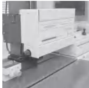
Surface roughness measuring machine
