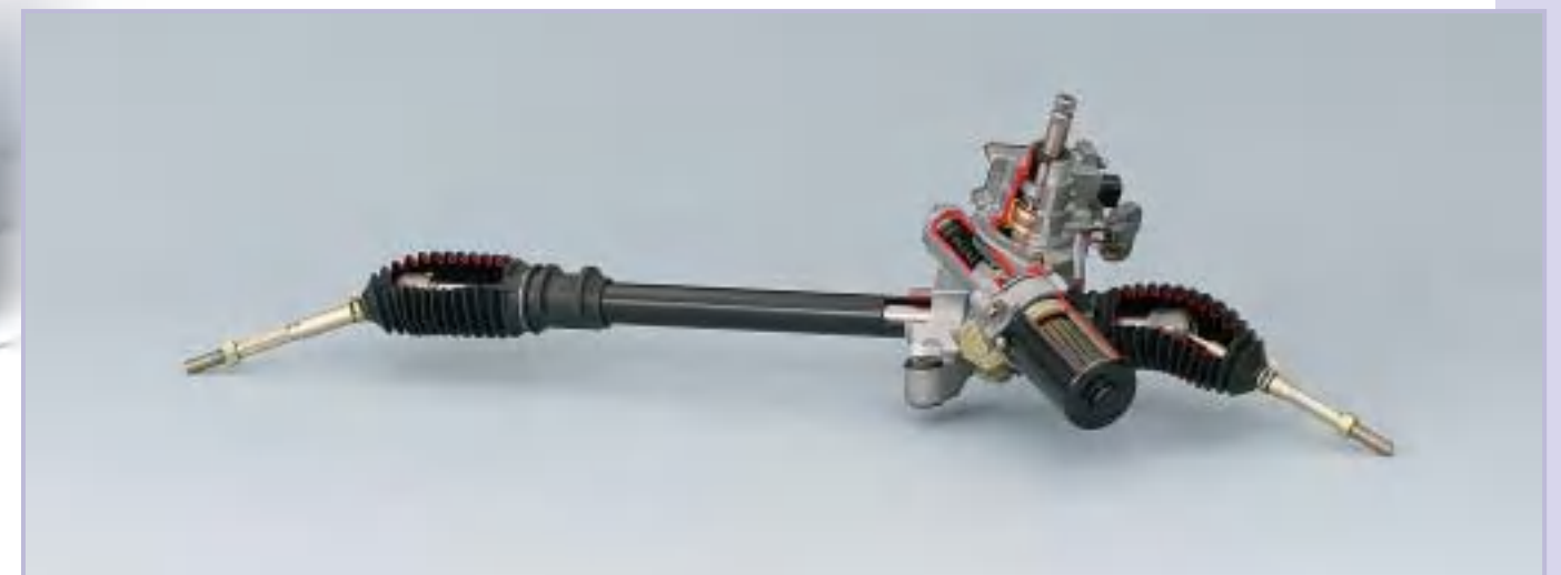
Pinion Type Electric Power Steering Pinion type EPS for small cars.
