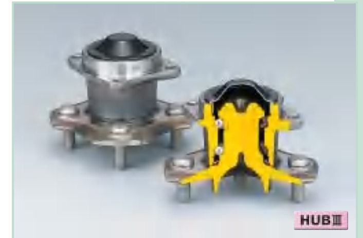
Double-Row Angular Contact Ball Bearings with Inner and Outer Mounting Flange (HUB III for Non-Driven Wheels) Double-row angular contact ball bearing with integral inner and outer mounting flange. Easy incorporation of ABS sensor.
