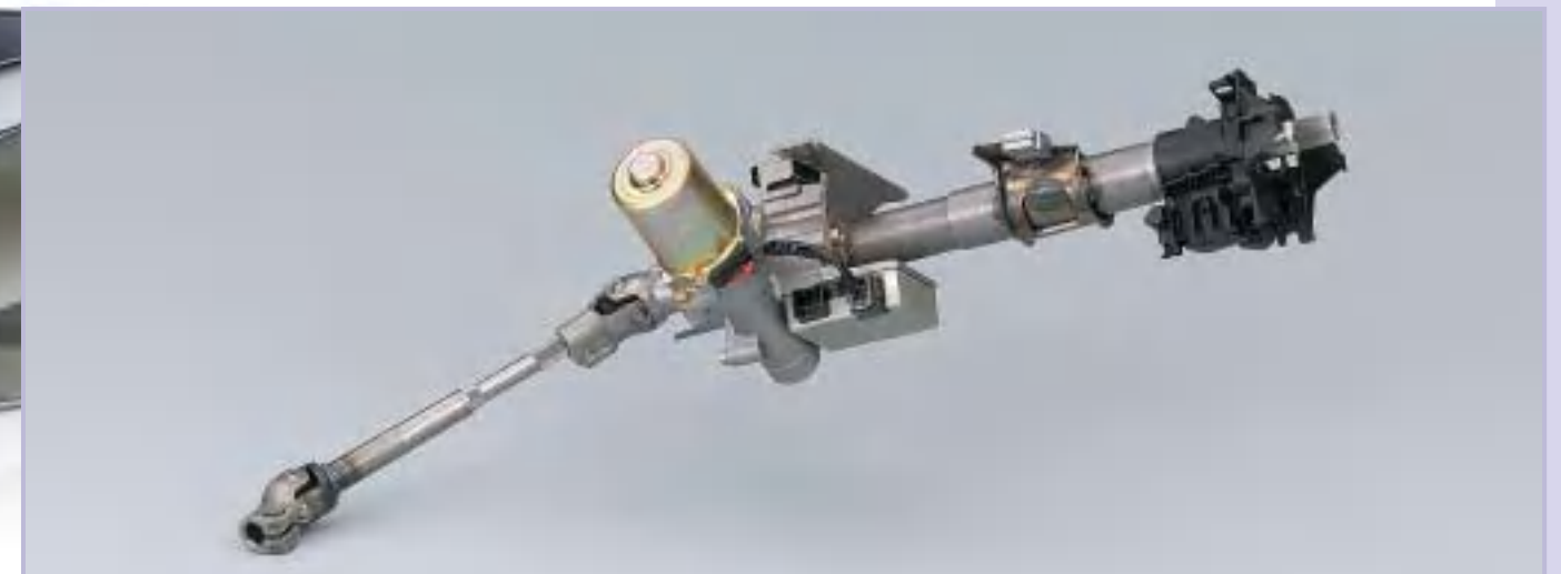
Column Type Electric Power Steering Column type EPS for minivehicles.
