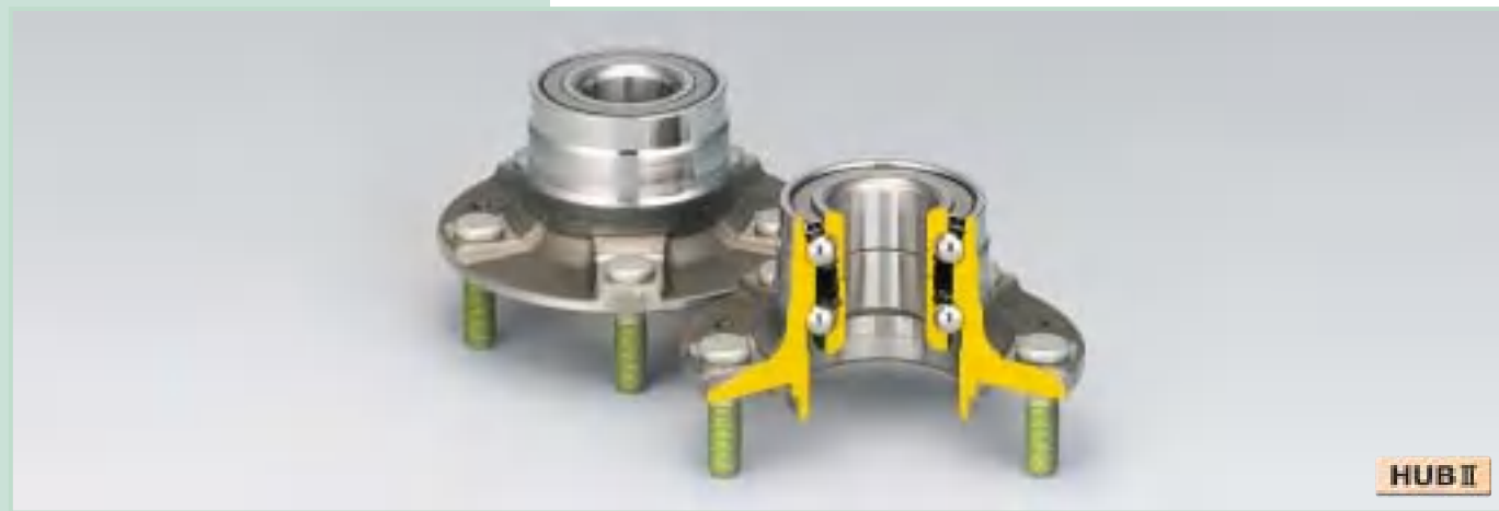
Double-Row Angular Contact Ball Bearings with Outer Mounting Flange (HUB II for Outer Ring Rotation Type) Outer ring rotating hub unit bearing with outer flange for mounting the wheel.
