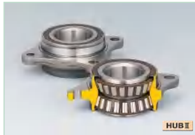
Double-Row Tapered Roller Bearings with Outer Mounting Flange (HUB II for Inner Ring Rotation Type) Inner ring rotating tapered roller hub unit bearing with integral flange for mounting onto knuckle. Suitable for heavy-duty vehicles.
