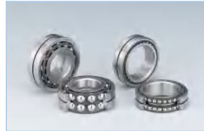
Long Life Double Row Angular Contact Ball Bearings Reduced weight and costs have been achieved by using PA46 plastic cage with superior oil and heat resistance. Initial internal clearance is used to provide optimum preload.
