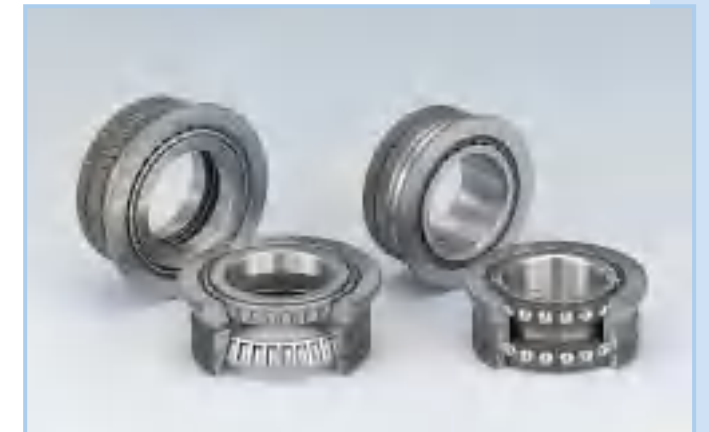
Long Life Double Row Bearings with Outer Ring Splines The outer ring has a mounting flange and splines, which attach to the one-way clutch. This affords greater compactness of FF-type automatic transmissions.
