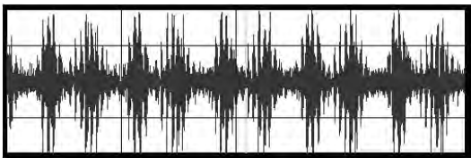
Sound waveform of a scratched bearing
