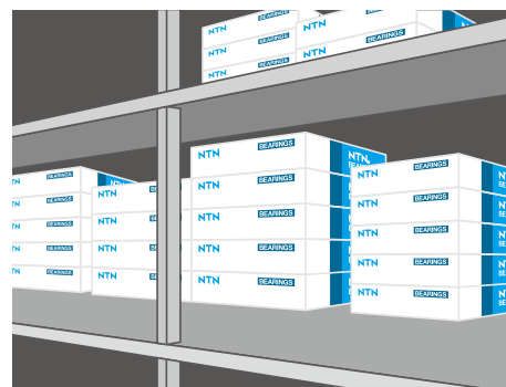
Fig. 15.4 Storing one-bearing boxes on a shelf
