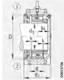
Design A Housing with Taconite seal
