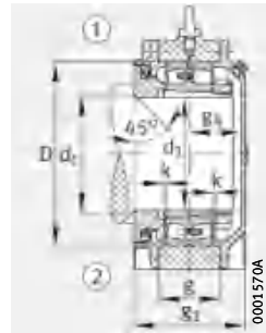
Design A Housing with Taconite seal
