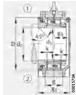
Design A Housing with Taconite seal
