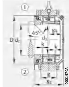
Design A Housing with Taconite seal
