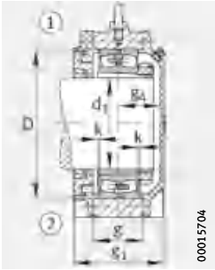
Design A Housing with labyrinth seal
