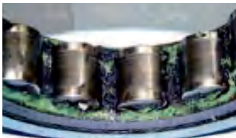
Lubricant degradation caused by electrical discharge currents
