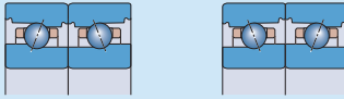
Static axial stiffness for two bearings arranged back-to-back or face-to-face – 719 .. B series
