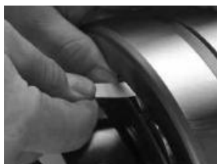
Fig. 14. Measure RIC before installation.
