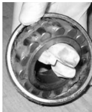
Fig. 21. Grease can easily be packed by hand.
